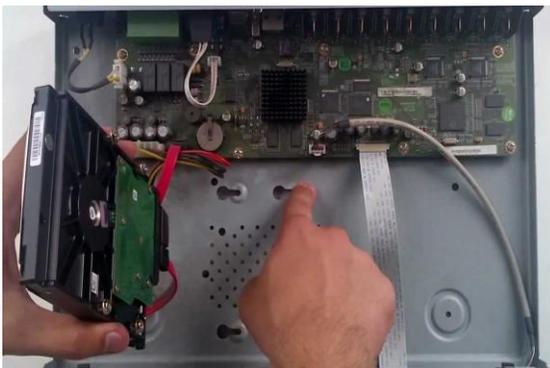
4) Turn the device upside down and then tighten the screws to hold the HD firmly in place.
