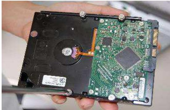
**3)** Line up the screws in the hard drive with the large holes in the bottom of the DVR, insert, and then move the HD so the screws are in the smaller area of the holes.
