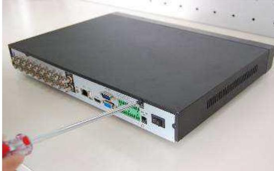
**2)** Loosely (a few turns) attach four screws (included) in the bottom of the HD.
