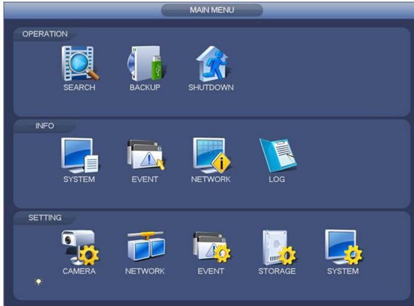
8) From the **Storage** screen (below) click on **HDD Manage** tab on the left. Under **SATA** you will see your HD listed (1, 2, 3, 4, etc. depending on how many drives installed). "O" means the drive is good, "-" means the drive is bad. The **HDD Manage** menu is a good place to return to check the health of your hard drive if problems show up in the future. That little "O" or "-" will tell you the health of your hard drive real fast.
